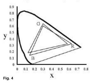
Equally important, since the primaries are at different locations, mixing the primaries with the same proportions of light will generate different colors. Hence we see that to reproduce the colors specified by video signals, it is critical that the primaries be matched to the video system standards.
